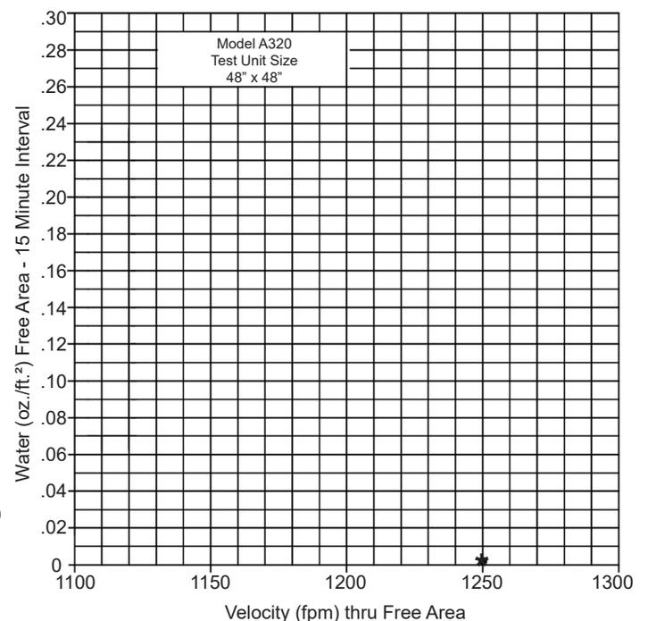
\* AMCA Standard 500 limits testing of Water Penetration to either a maximum velocity of 1250 FPM or 2.5 ounces of water per square foot of louver Free Area.
