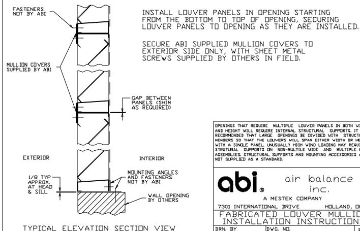
OPENINGS THAT REQUIRE NULTIPLE LOUVER PANELS IN BOTH WIDTH AND HEIGHT WILL REQUIRE INTERNAL STRUCTURAL SUPPORTS, IT IS RECOMMENDED THAT LARGE OPENINGS BE DIVIDED WITH STRUCTURAL MEMBERS SO THAT THE LOUVERS WILL SPAN EITHER WITH STRUCTURAL WITH SINGLE PANEL UNUSUALLY HIGH WIND LOADING MAY REQUIRE STRUTURAL SUPPORTS ON NON-MULTILE WIDE AND MULTIPLE HIGH ASSEMBLIES, STRUCTURAL SUPPORTS AND MOUNTING ACCESSORIES ARE NOT SUPPLIED AS A STANDARD.
