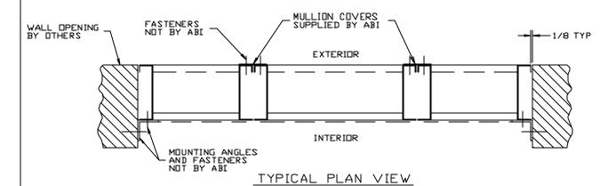
INSTALL LOUVER PANELS IN OPENING FROM LEFT TO RIGHT AS VIEWED FROM INTERIOR OF OPENING AND SECURE TO OPENING.
