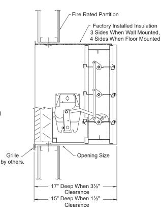
Combination Fire/Smoke Damper ▲ 1½ Hr. Rated ▲ Single Thickness Blades ▲ Leakage Class II ▲ 250°F or 350°F Rated ▲ Front Access Grille ▲ Galvanized Steel
