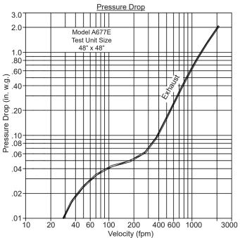
Exhaust air converted to .075 lb./cu.ft. air density.
