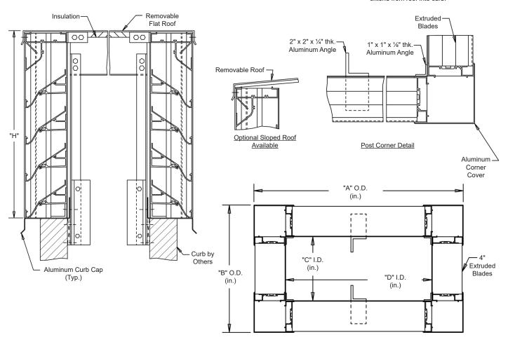
Continuous angle at the four corners and intermediate as required.
